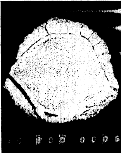
Fig. 3. A cross section of the positive grid of a lead–acid battery showing corrosion and spallation of the corrosion layer.
